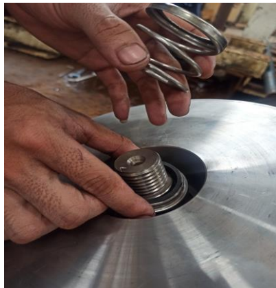
Gambar 4. 20 Pemasangan Mechanical Seal Stationary (Sumber: dokumen pribadi)
