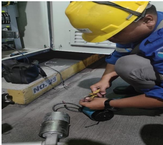
Gambar 2. 29 Test Motor Vale Compressor PG 2 (Sumber: Dokumentasi di PT. Indah Kiat Pulp and Paper)
