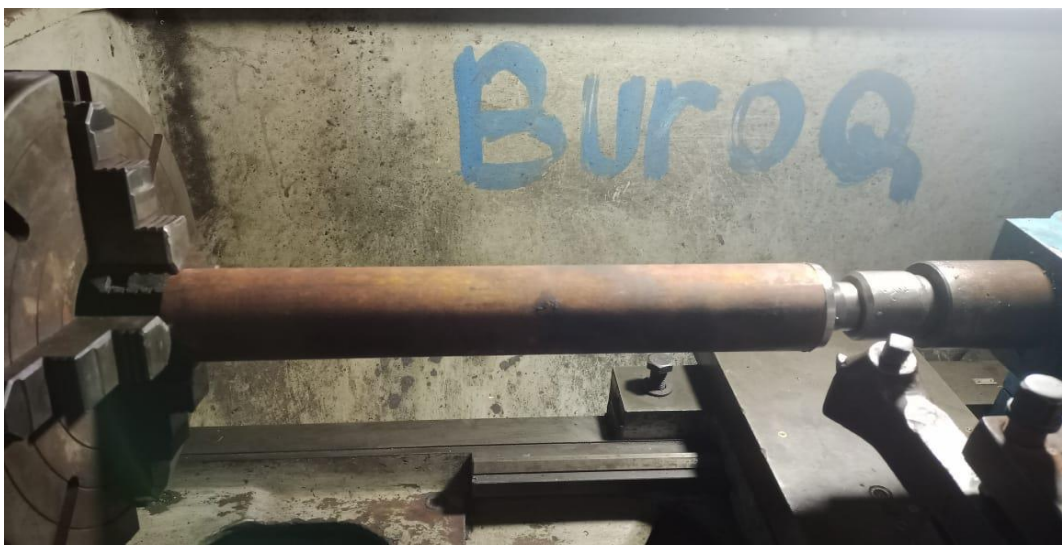
Gambar 3.6 pembubutan as Transfer Carriage
