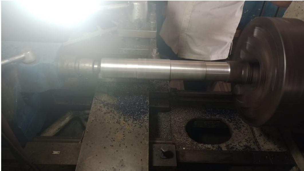
Gambar 3.8 pembuatan as Transfer Carriage
