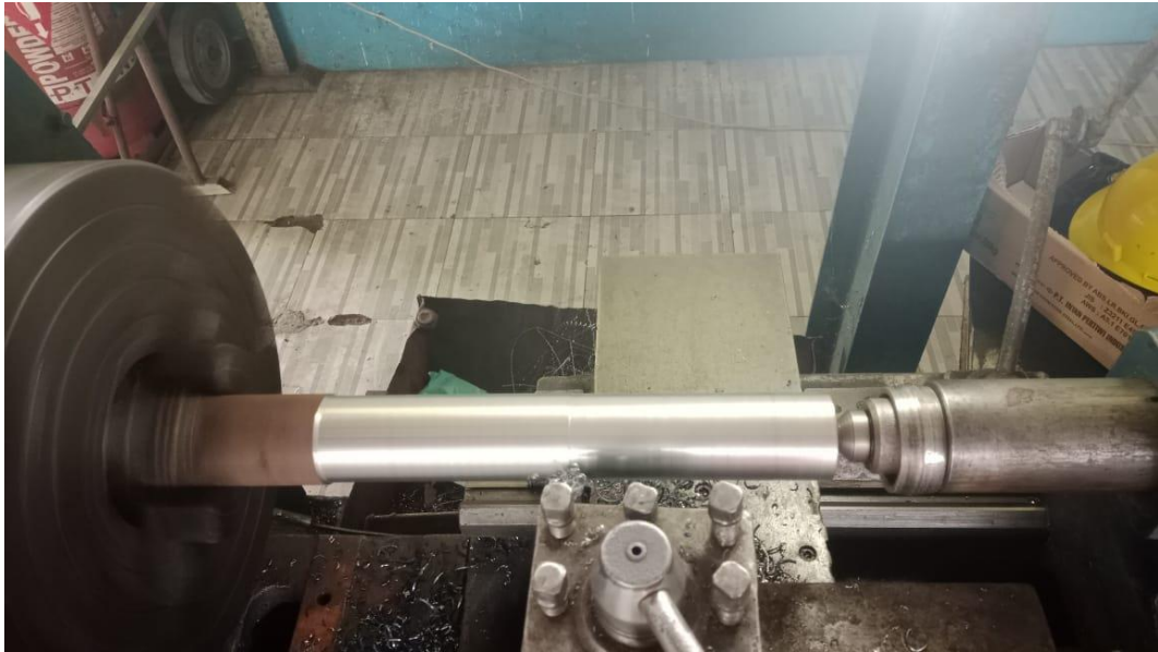
Gambar 3.1 pembubutan as Transfer Carriage
