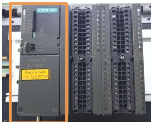
Gambar 3. 2 CPU Siemens S7-300
