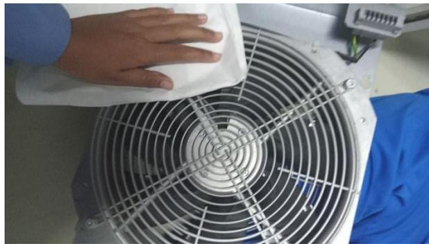
Gambar 3. 21 Gambar *Cleaning Fan Drive*
