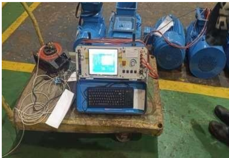
Gambar 3. 1 alat static motor analyzer awaiv-12kv
