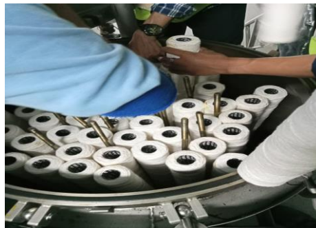
Gambar 2. 17 Repair Filter Catridge (sumber: dokumentasi pribadi)
