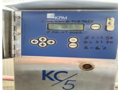
Gambar 2. 5 Transmitter consistency PT. Invenus
