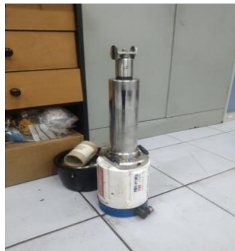
Gambar 3. 3 Sensor Consistency KPM KC/5
