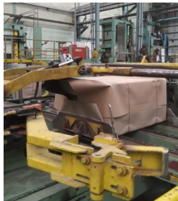
Gambar 3. 6 Folding Machine melipat sisi bawah (Sumber: PT. Riau Andalan Pulp and Paper )
