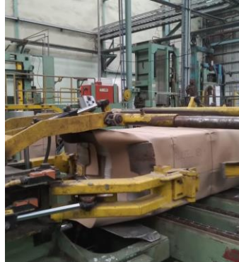
Gambar 3. 5 Folding Machine melipat sisi samping (Sumber: PT. Riau Andalan Pulp and Paper )
