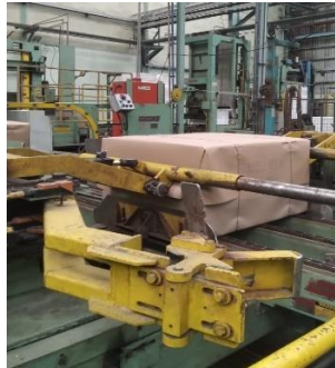
Gambar 3. 7 Folding Machine melipat bagian atas (Sumber: PT. Riau Andalan Pulp and Paper )
