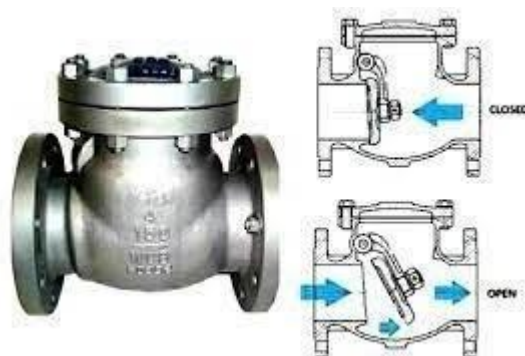
Gambar 4.16 Swing Check Valve (Sumber : www.google.com )
