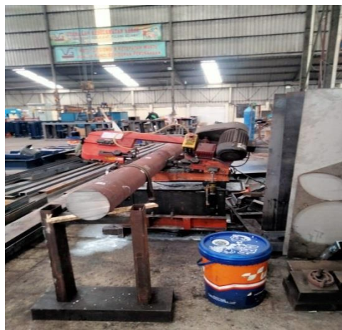
Gambar 4.3 proses pemotongan bahan drive shaft wy p20 short
