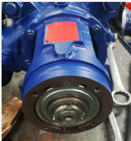
Gambar 4.28 Pemasangan Bearing House Section
