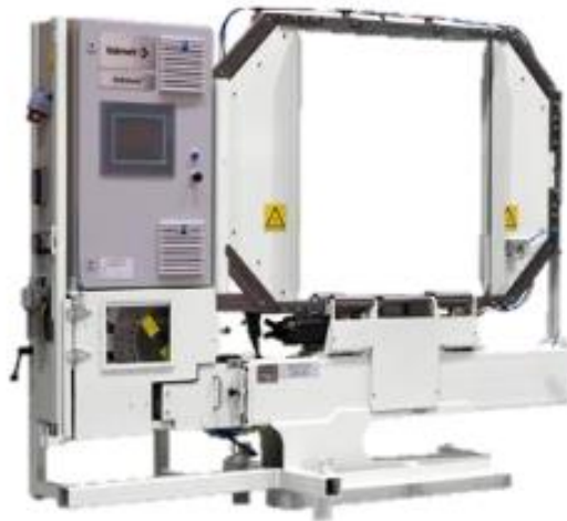
Gambar 3. 2 Tying machine (Sumber: Dokumentasi PT. Riau Andalan Pulp and Paper Pangkalan Kerinci, 2023)
