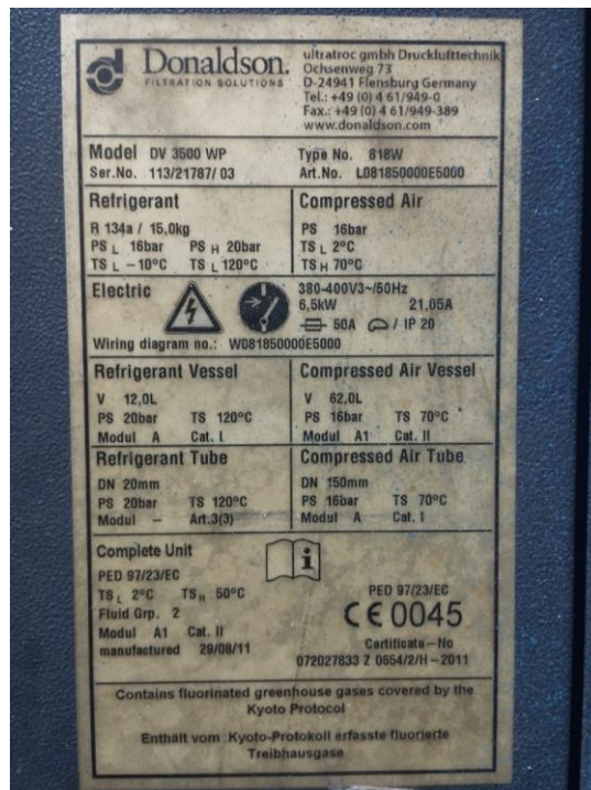
Gambar 4. 25 Nameplate air dryer
