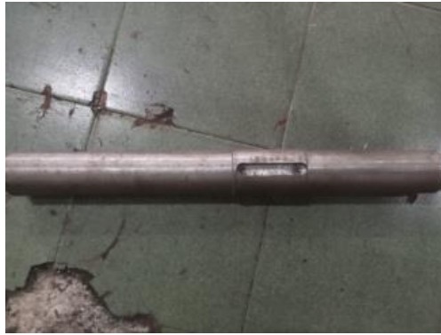
Gambar 4. 16 shaft transfer carriage Sumber : Dokumentasi
