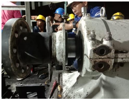
Gambar 4. 15 Pelepasan cover koupling
