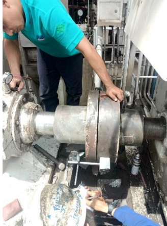
Gambar 4. 17 Pengambilan data alignment
