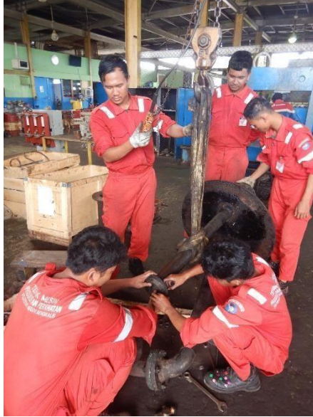
Gambar Lampiran 1: Maintenance Vertikal Sump pump
