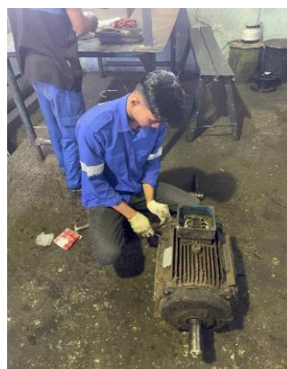
Gambar 2. 37 Mencopel elmots 22kw
