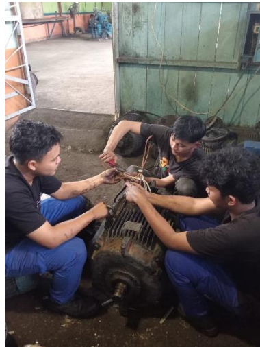
Gambar 2. 68 Mencopel elmots 55 kw
