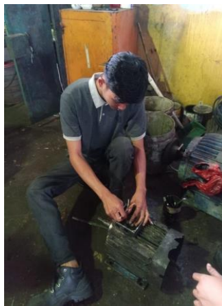
Gambar 2. 26 Mencopel elmots conveyer 7,5 kw
