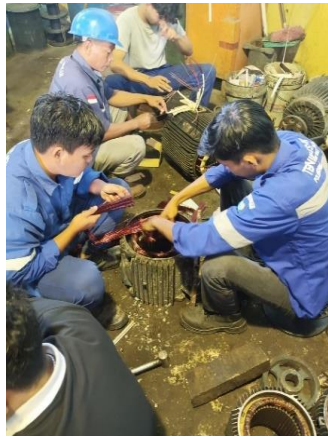
Gambar 2. 50 Mencopel elmots 15 kw
