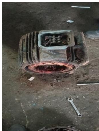
Gambar 2. 24 Mencopel elmots 22 kw
