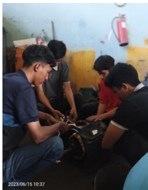
Gambar 2. 10 Mencopel elmots 22kw
