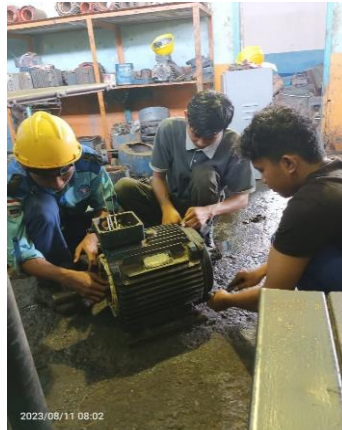
Gambar 2. 54 Mencopel elmots 15 kw
