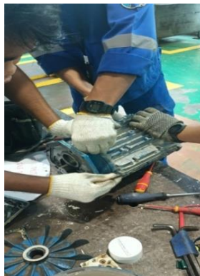
Gambar 2.14 Penggantian Bearing Motor 3 Fasa 4 kw
