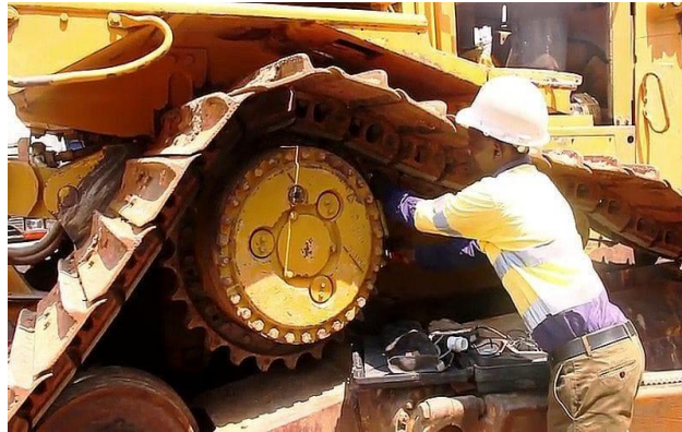
Gambar 4.22 Track Link (Sumber: PT. Vadhana International )
