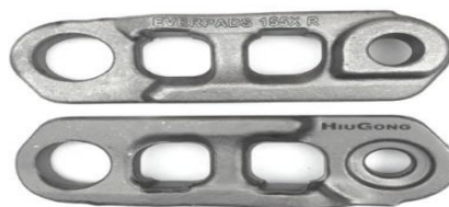
Gambar 4.12 Track Line Joint (Sumber: PT.Vadhana International)
