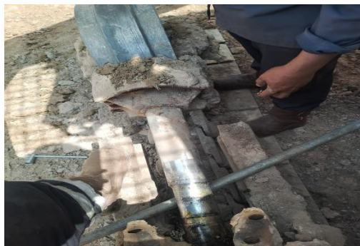
Gambar 4.20 Lepas as dan idler dozer (Sumber: PT. Vadhana International)
