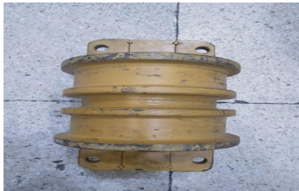
Gambar 4.14 Track Roller (Sumber: PT.Vadhana International)
