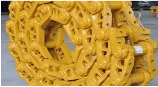
Gambar 4.10 Track Line (Sumber: PT.Vadhana International)
