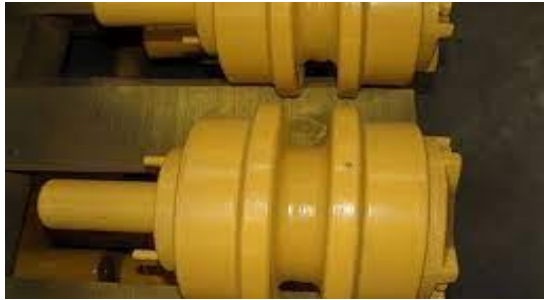
Gambar 4.15 Carrier Roller (Sumber: PT.Vadhana International)
