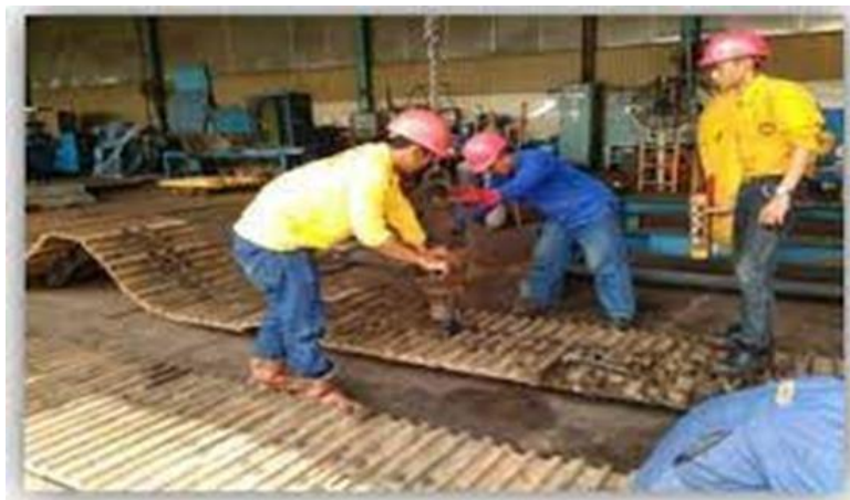
Gambar 4.21 Track Shoe Dozzer (Sumber: PT. Vadhana International)
