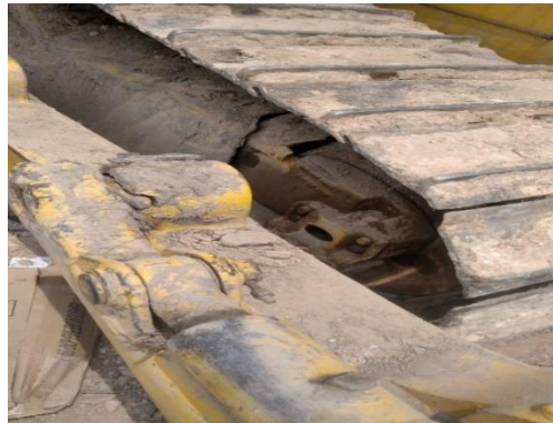
Gambar 4.17 Idler Buldozer (Sumber: PT.Vadhana International)
