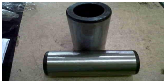
Gambar 4.11 Track Bushing (Sumber: PT.Vadhana International)
