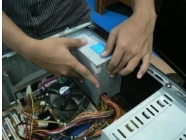
Gambar 3.12 Memasang Power Supply
