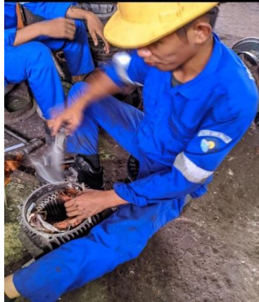
Gambar2. 68 Membongka motor conveyor
