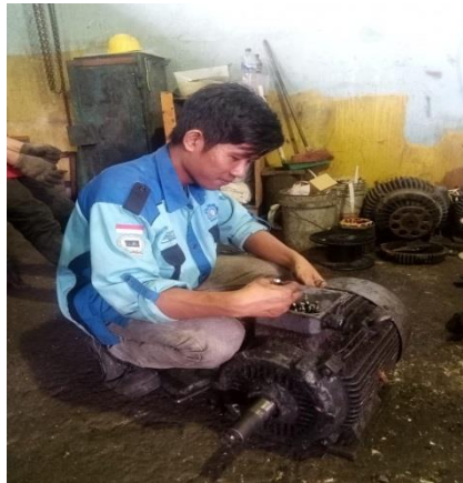
Gambar2. 47 Masang star dan delta motor ripple mill
