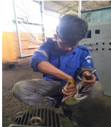
Gambar2. 59 Membongkar motor conveyer
