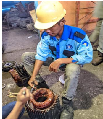
Gambar2. 27 membongkar motor crane
