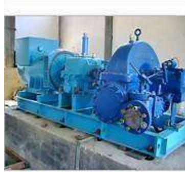
Gambar 4. 1 Turbin Uap single steam :www.tradeindia.com
