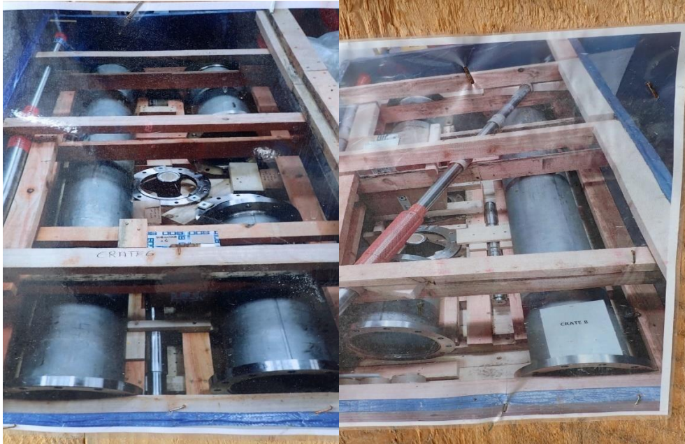
Gambar 4.6 Impeler Suction Fire Pump 717-PE-3
