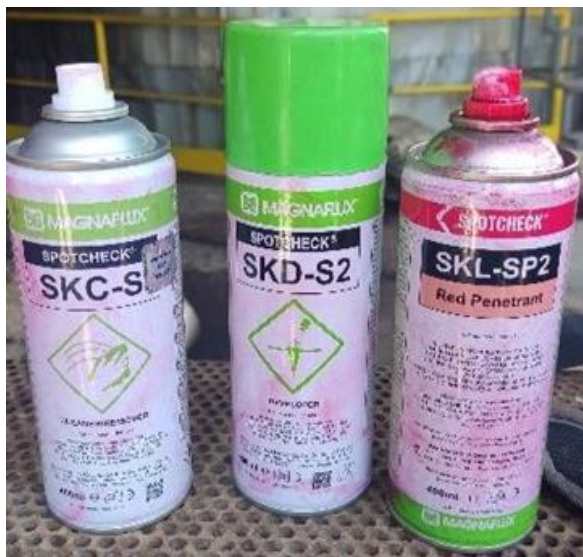
Gambar 4. 4 Cairan Penetrant Test sumber: PT RAPP
