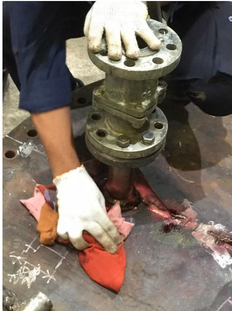
Gambar 4. 8 Pembersihan Sisa Red Penetrant Sumber : Workshop PT. RAPP
