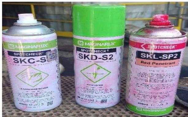
**Gambar 3. 9 Cleaner, Penetrant & Developer**
