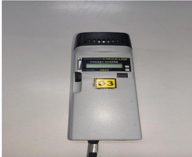
**Gambar 3.1 Stroboscope**
