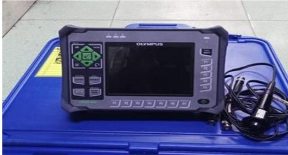
**Gambar 3.12 Ultrasonic Testing (UT)**
