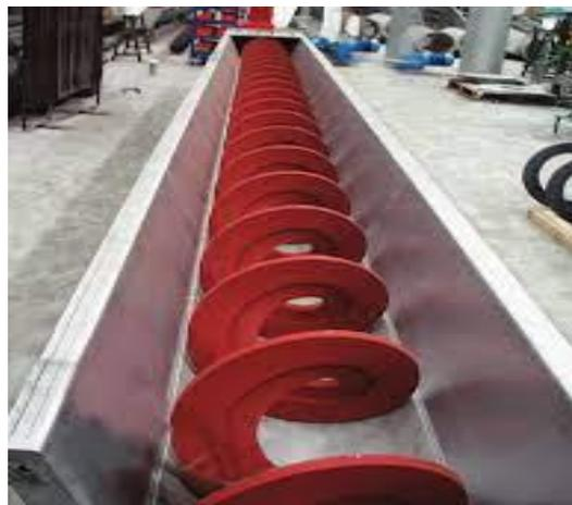
**Gambar 4.5 *Shaftless Screw Conveyor***
