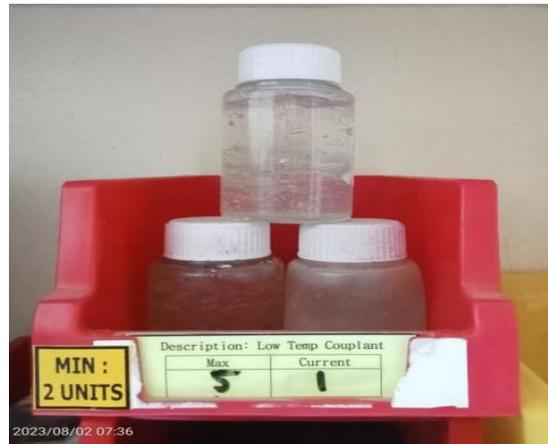
**Gambar 3.16 ultrasonic couplant gel (UTG)**
