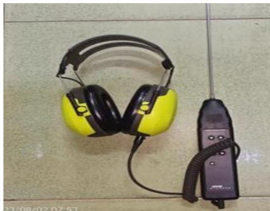
**Gambar 3.15 stetoscope**
