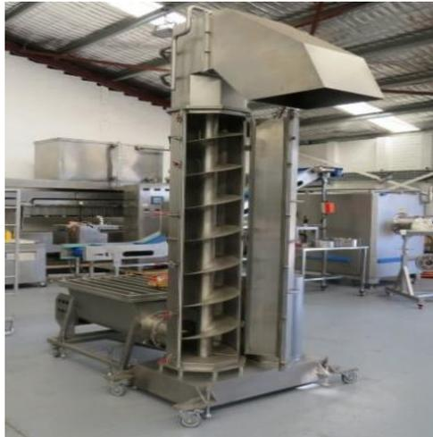
**Gambar 4.6** *Vertical Screw Conveyor*
