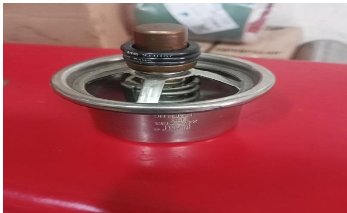
Gambar 4. 7 Regulator/Thermostat (Sumber : Dokumentasi Pribadi)
