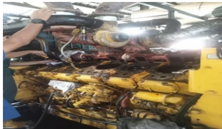
Gambar 2.14 Kegiatan servis unit lima (Sumber: PT. Megapower Makmur Tbk, 2023)
