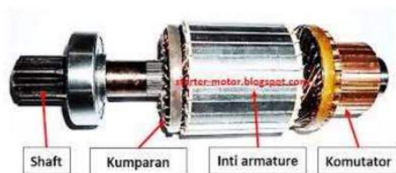
Gambar 3.12 : Armatur Shaft. (Sumber : https://images.app.goo.gl/H4YYa4oA2xZL7nyL9 ).
