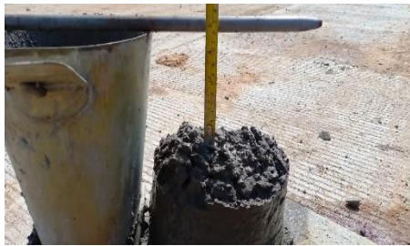
Gambar 4. 13 proses pengujian slump beton
