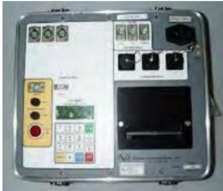
Gambar 3.15 Breaker Analyzer Sumber: (Brist, 2023)
