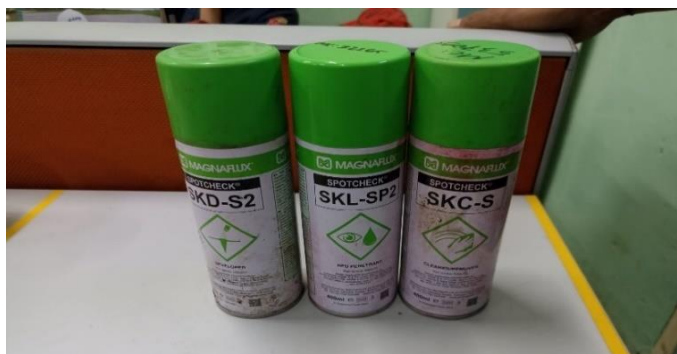
Gambar 3.9 Cleaner, Red Penetrant & Developer Sumber: Como RPL Office, PT. RAPP
