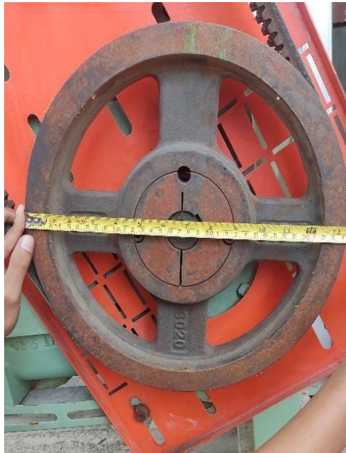
Gambar 4.21 Pengukuran diameter pulley Sumber: PT. RAPP
