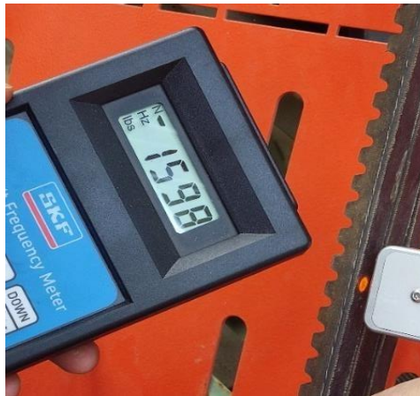
Gambar 4.28 Cek ketegangan v-belt Sumber: PT. RAPP
