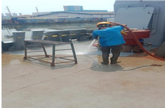
Gambar 3. 6 Proses Hose test
