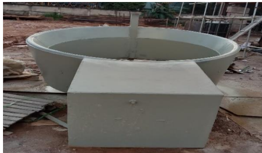
Gambar 3.22 finishing kort nozzle
