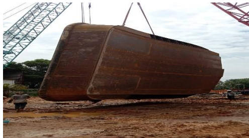
Gambar 2.121 Erection buritan kapal tug boat hull 08
