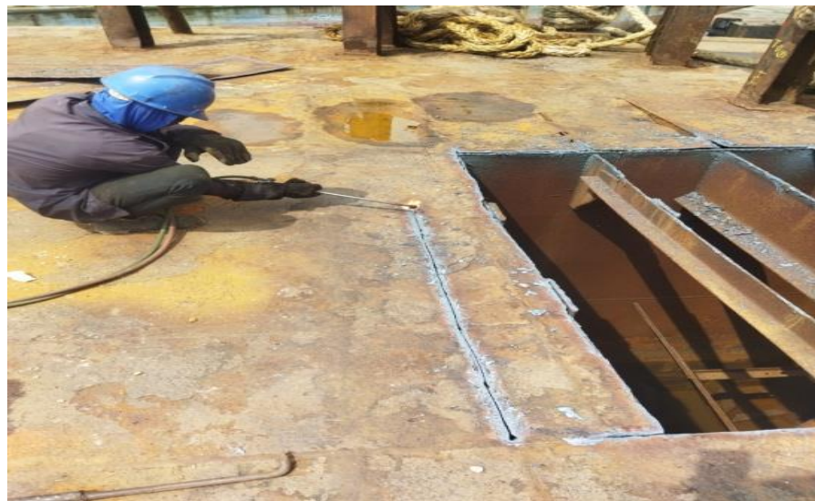
Gambar 2.28 cutting di main deck tongkang frame 32
