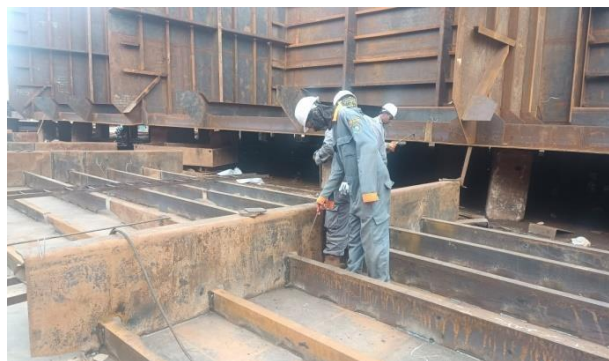
Gambar 2. 62 Inspect welding terhadap side shell
