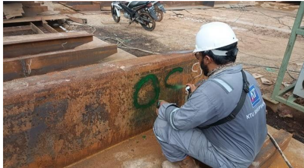
Gambar 2. 55 Proses penandaan panel main deck
