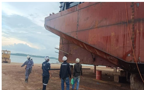
Gambar 2. 64 Proses air pressure test eksternal
