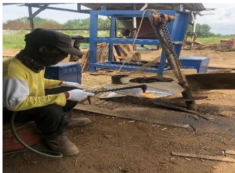
Gambar 2 22 Proses penambalan propeller
