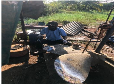
Gambar 2 25 Proses penambalan propeller
