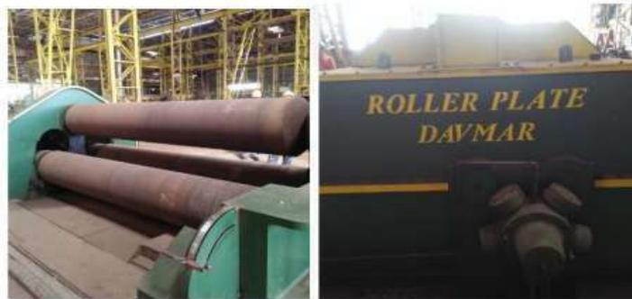
**Gambar 1.4 Mesin *Rolling***
