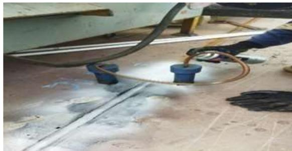
**Gambar 2.45** pengujian MPI
