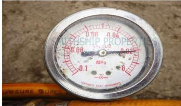
**Gambar 2.25 Vacuum Pressure Gauge**
