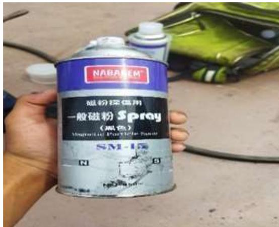
**Gambar 2.48** *Magnetic Particle Spray*
