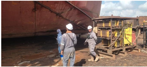
Gambar 2. 51 Air Pressure Test kapal tongkang
