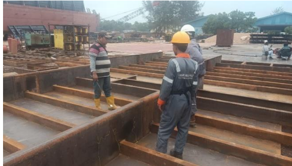
Gambar 2. 7 Inspect welding terhadap Transverse Bulkhed
