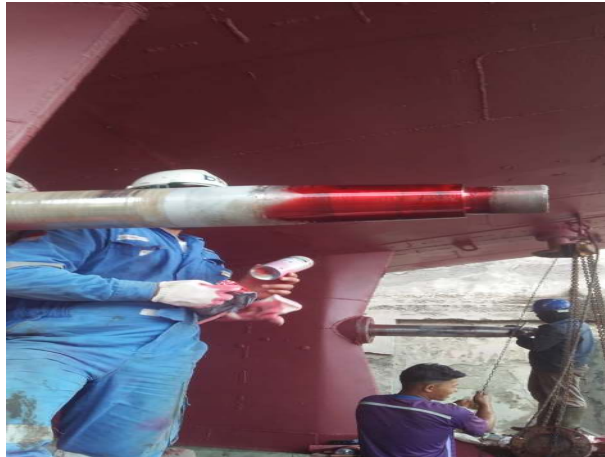
Gambar 2.17 Propeller Shaft Saat Uji Penetrant
