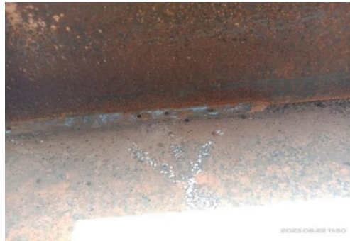
Gambar 1. 60 contoh cacat welding porosity
