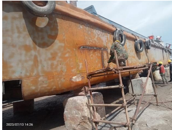
GAMBAR 2. 6 replating bodi kapal
