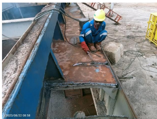
GAMBAR 2. 32 replating main deck kiri
