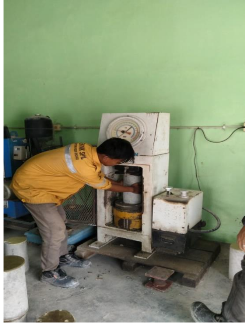
Gambar 3. 5 Uji kuat tekan sample beton
