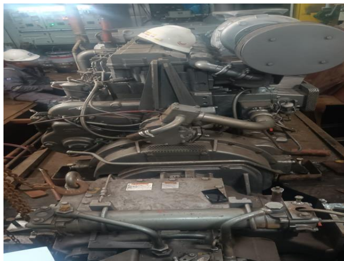
Gambar 2. 12 proses pemasangan gearbox kapal tug boat
