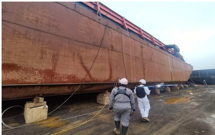
Gambar 2.56 air tast external
