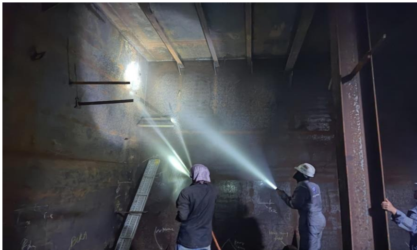
Gambar 2. 54 air tast tengki kapal hull 1645
