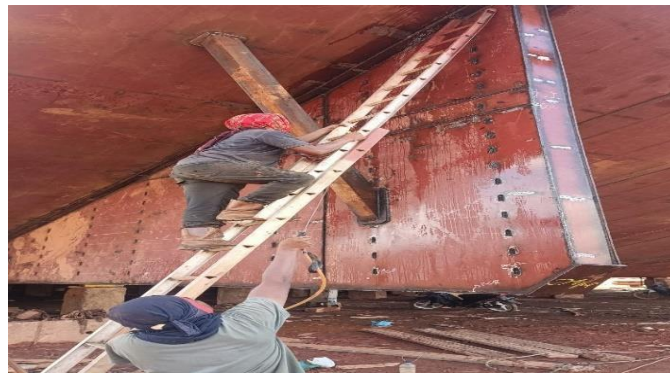
Gambar 2. 35 Proses air pressure test skeg
