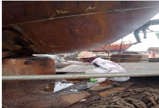
Gambar 2. 59 Penetran Test TB Indopower
