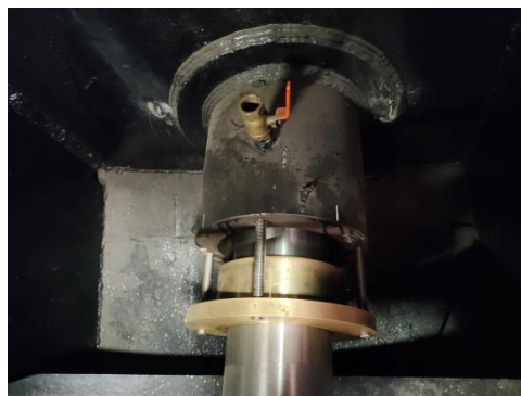
Gambar 3. 11 Pemasangan Kopling AS Propeller
