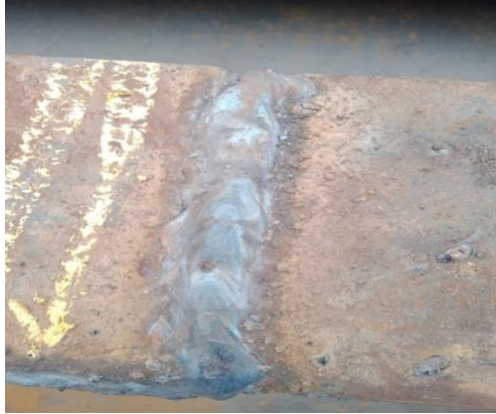
Gambar 2. 5 Cacat Las Overlap
