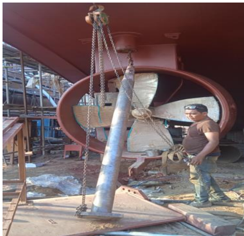
Gambar 5.11 Pemasangan as kemudi
