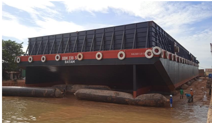
Gambar 2.24 Proses launching cargo deck barge
