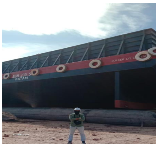
Gambar 2.22 Proses launching cargo deck barge
