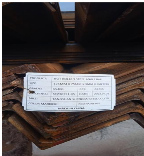
Gambar 4.16 Pengecekan ukuran Eagle
