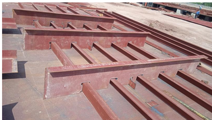
Gambar 3.9 Pengecekan Fit-up L.bhd
