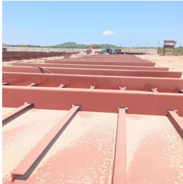
Gambar 2.107 Gambar bagian L.bhd belum cleaning
