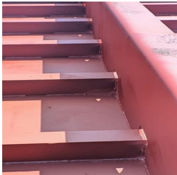
Gambar 2.102 Gambar hasil paintingan T.bhd hull 024
