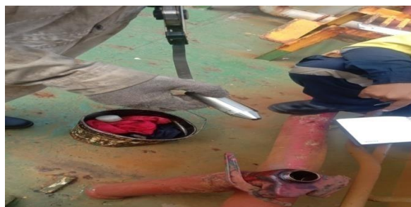
Gambar 2.24 loading survei (sounding pipe)
