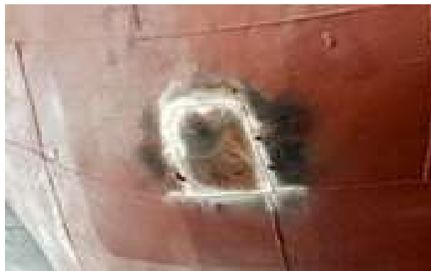
Gambar 2.143 Hasil Penetran Test Kamar Store
