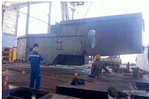
Gambar 2.37 Control Pemindahan Deck House T.036 Louis Dolphin
