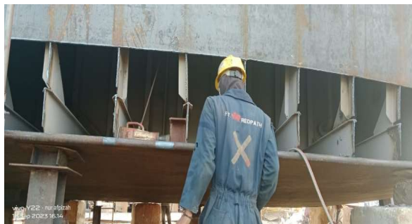
Gambar 2.60 Inset plate side shell T.033 Jx Walrus
