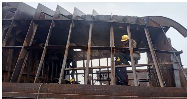
Gambar 2.66 Control Fiting web T.037 Grando Dolphin
