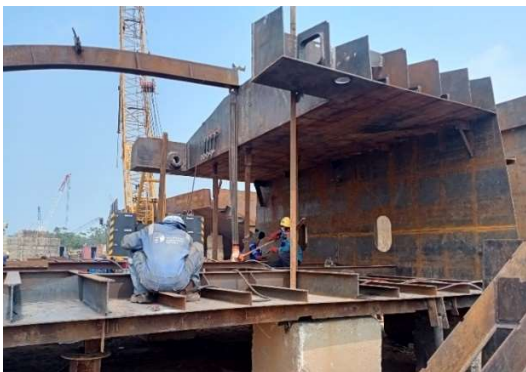
Gambar 2.62 Control Fitting keel T.037 Grando Dolphin
