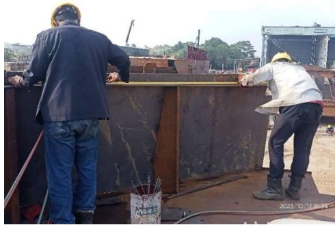
Gambar 2.82 Control Fitting Bulwark T.033 Jx Walrus
