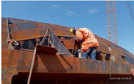
Gambar 2.29 Control Grinding Web AFT Kapal Multicat Jx Walrus T.033
