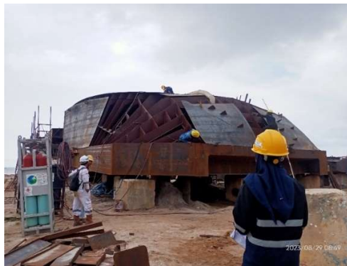
Gambar 2.45 Control Instal Kulit Bottom T.033 Jx.Walrus
