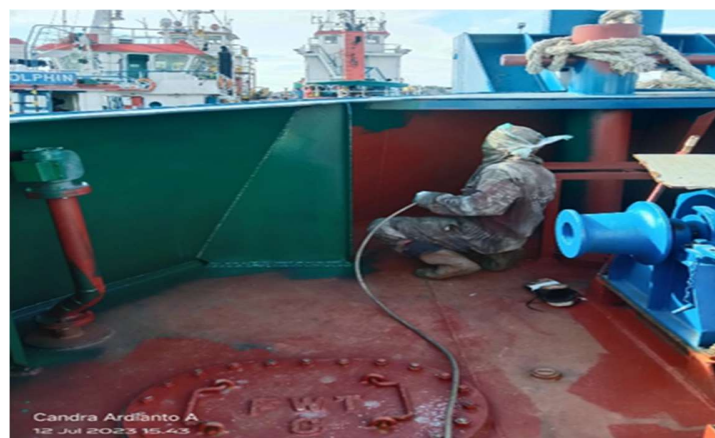
Gambar 2.8 Control proses painting bulkwalk T.027 Marino dolphin
