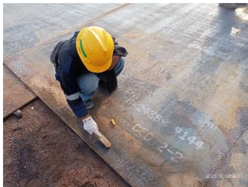
Gambar 2.85 Tracing material Main deck T.034 Jx Silion
